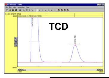
This chromatogram is from a direct injection of 0.5mL of human breath. The longer we hold our breath, the higher the  $CO_2$  content. This was the result of a class experiment called "Waiting to Exhale," which is included in the manual. It is a contest to see who can blow the most  $CO_2$ . Participants merely exhale into a 3mL syringe, then inject 0.5mL into the on-column injector of an Educational TCD GC.
